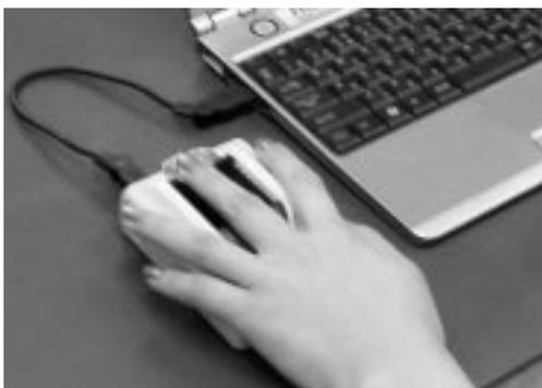
Hitachi focused on the finger vein. If a couple of fingers are registered, even when a person injured a finger, the system can still authenticate him. Each person registers his fingers, and a computer authenticates him by comparing the registered data and the fingers. This basic technology was developed in 2000, and it was commercialized and applied to the door-access-control for computer rooms in 2002.
